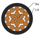
Bare copper conductor LSOH rubber compound insulation
